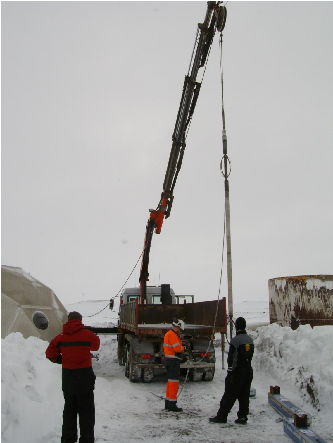
Figure 1. Natural gamma ray instrument with in-line centralisers being prepared for a demonstration run up to 300°C.
