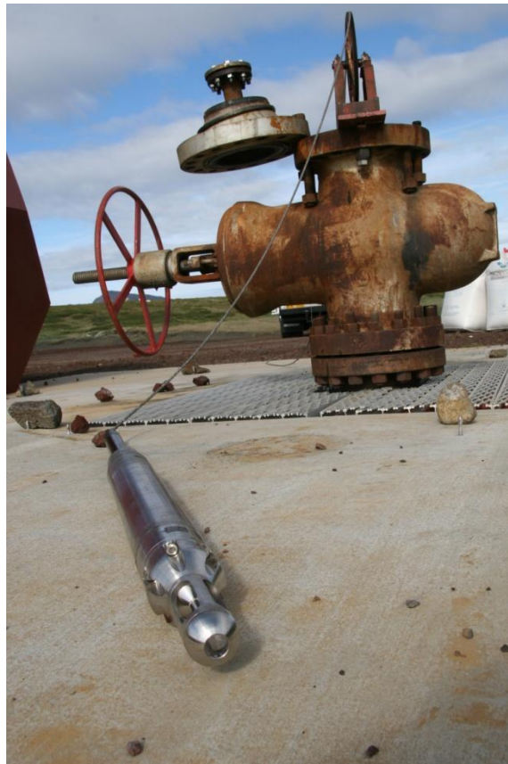
Figure 1. BRGM temperature tool before going into a high temperature well at Krafla
